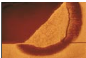
Cracked welds pose danger. This weld joint in low-alloy steel cracked because it did not cool properly.
